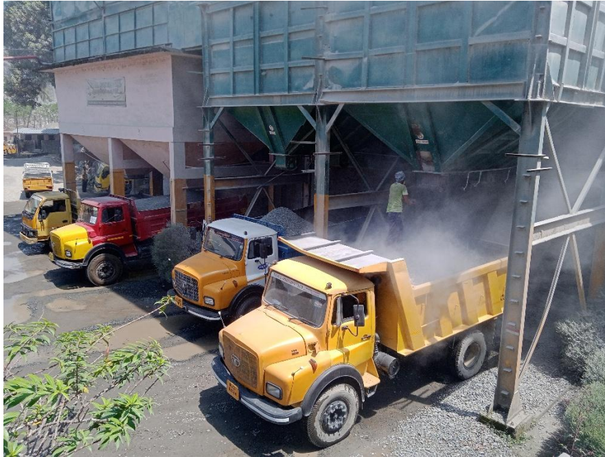
Figure 12: Tipper trucks collecting sand from a crusher in the Western Ghats (credit: Author)
