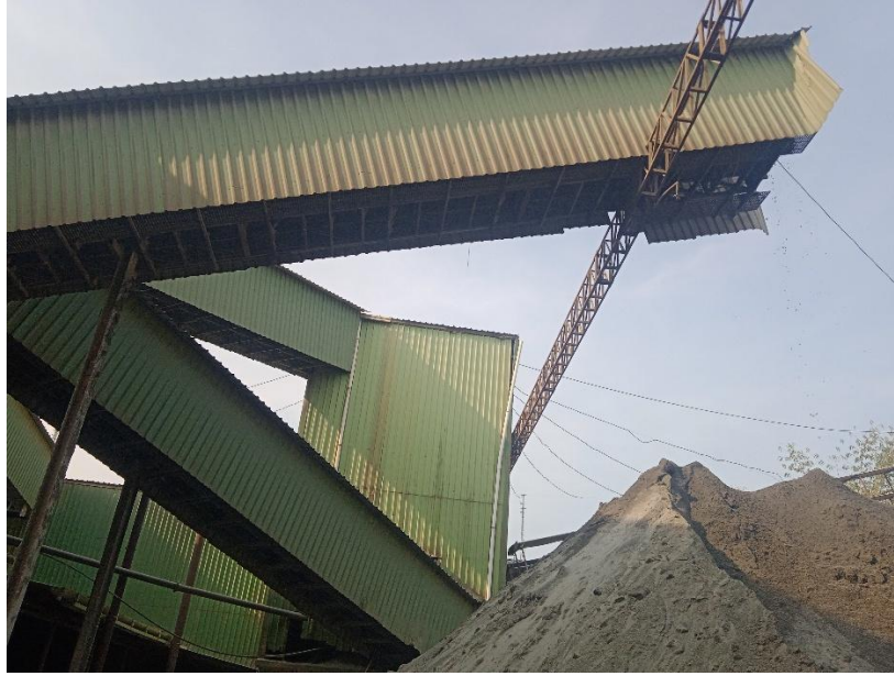
Figure 11: Crusher producing m-sand in the Western Ghats (credit: Author)
